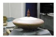
The base was remounted in the chuck, the lid fitted and the tailstock brought up to hold the lid in place. Using gentle cuts the lid was shaped to follow and blend in with the gentle curve of the top of the base. Mike used the scraper to remove the tool marks and sanded to finish. A shallow hole was drilled in the centre of the lid and a previously turned finial fitted.
